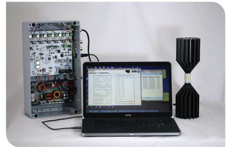
Shown with the Universal LED Controller, the light source is easily programmable using Sealite's PC Configuration Tool
