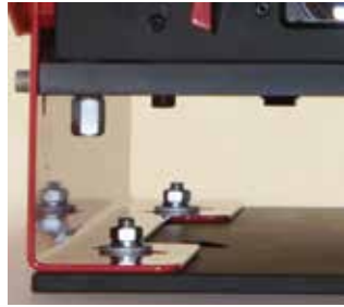
Pedestal Three prolonged \varnothing 16 mm mounting holes on a 200 mm circle.
