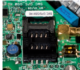
Remote monitoring GSM unit and antenna integrated in the lantern for remote monitoring and control. For more information, please see the LightGuard Section.
